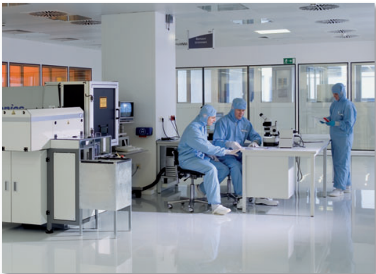
Temperature sensor production under clean room conditions
